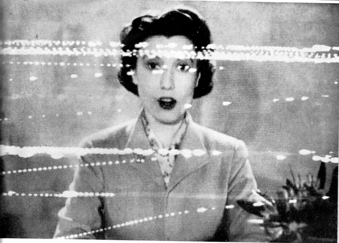
FIG. 2—IGNITION INTERFERENCE WITH TELEVISION RECEPTION.
