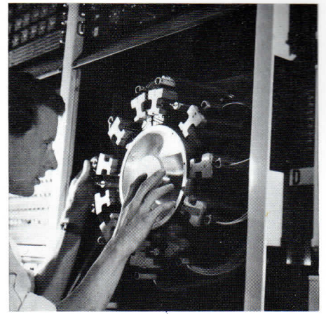
Magnetic drum register-translator: one of the magnetic drums which determine the routes to be taken by calls from London over the network of circuits to all parts of Britain.
