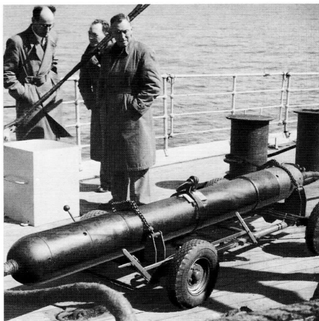
FIG. 6—Dollis Hill engineers (Messrs. V. G. Welsby, E. F. S. Clarke and R. A. Brockbank) on the deck of cable ship Monarch during submarine repeater laying trials in 1954
