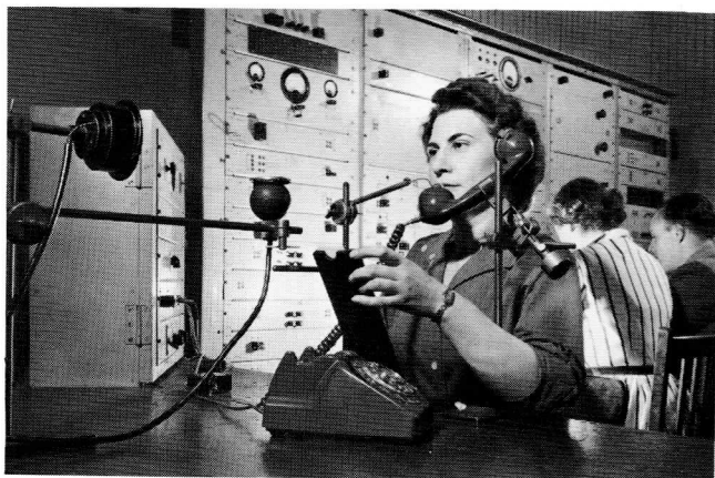
FIG. 7—Speech tests on a prototype 700-type telephone in 1958
