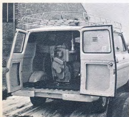
A large order supplied to Korea included the provision of an independent power supply. Shown here is the generator van, supplied by Pye TVT for this purpose.
